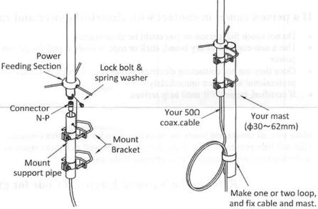
Note: For long-term use, water-proofing with glue, self-fusing tape, and/or vinyl tape is highly recommended.
