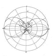
Elevation pattern: This pattern represents the typical elevation pattern when the GP-15 is mounted in free space without interference from other metal objects. The inner most lobe is the 440MHz elevation pattern, the largest lobe is the 6M elevation pattern. The lobe between is the 2M elevation pattern.
